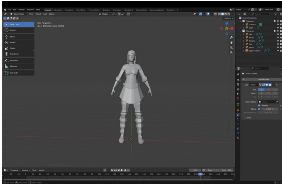
Figure 1: Mirror modifier configured on the upper clothes object: mirroring across the X axis, with clipping enabled and a 1 mm merge threshold.
